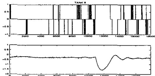
Fig. 6. Top: Control action sent by Controller, Bottom: Level Measurement
