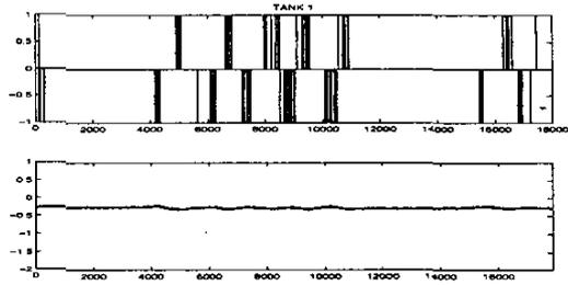
Fig. 4. Top: Control action sent by Controller, Bottom: Level Measurement
