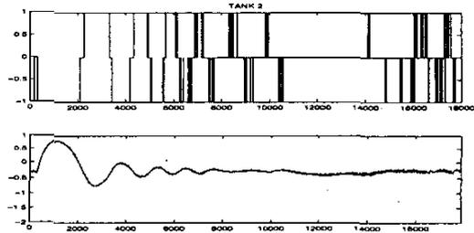
Fig. 5. Top: Control action sent by Controller, Bottom: Level Measurement
